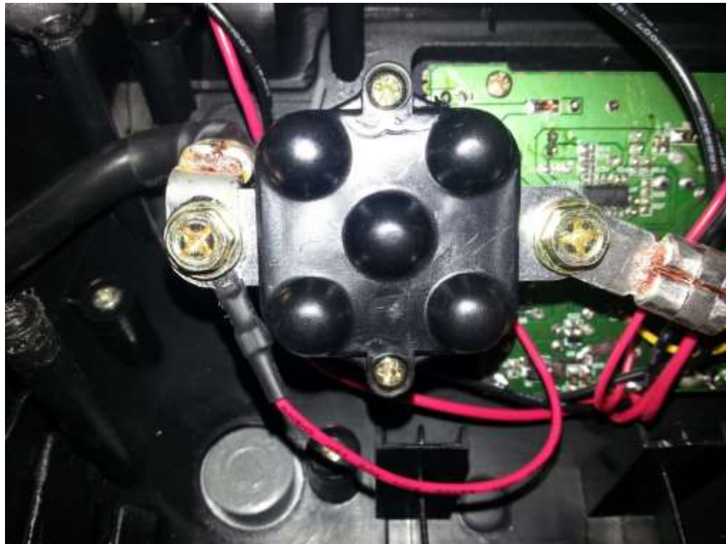
Fig. 155 - Attaching wires to the on/off control mechanism
