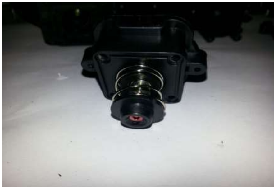
Fig. 133 - Inserting the spring and shaft into the housing
