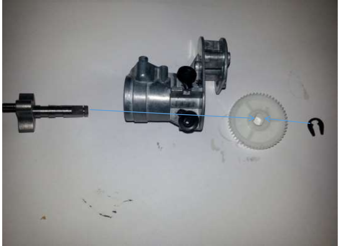
Fig. 116 - Assembling the lower portion of the compressor
