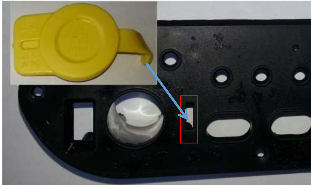
Fig. 142 – Inserting outlet cover
