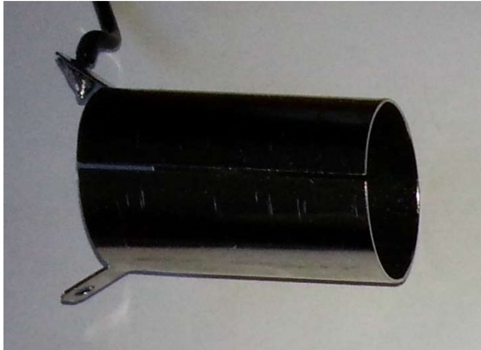
Fig. 138 – Solder wire to the DC cylinder
