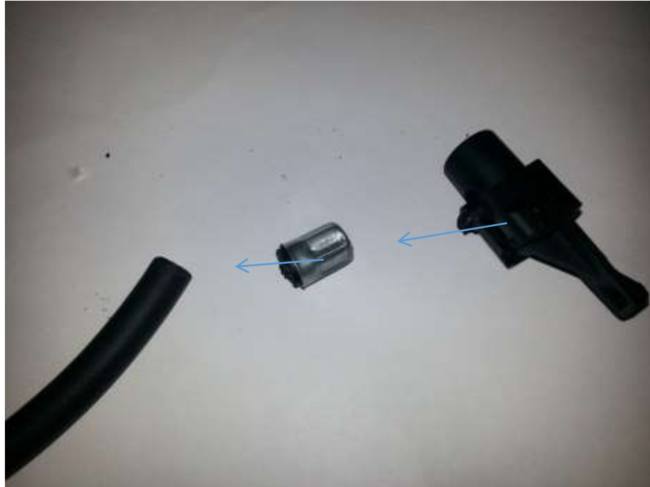
Fig. 96 - Attaching the valve to the hose
