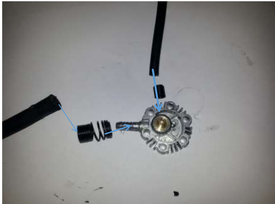
Fig. 113 - Attaching the valve and pressure gauge hoses to the compressor top
