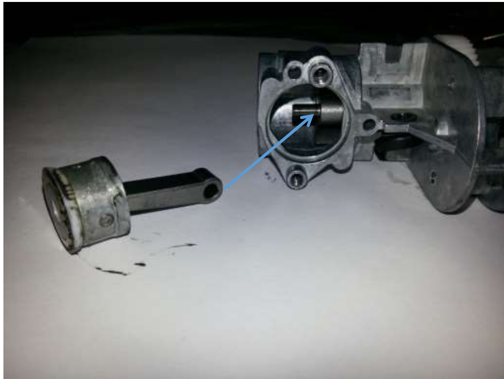
Fig. 120 - Attaching the piston to the cam
