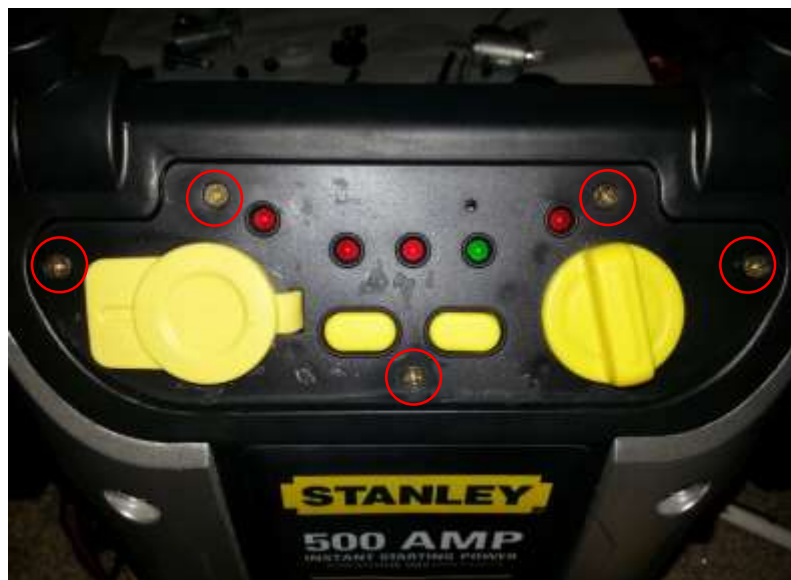
Fig. 153 - Attaching the front panel to the housing
