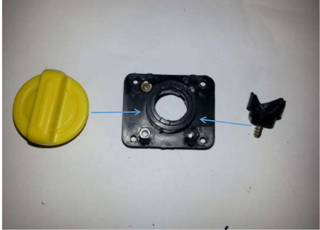
Fig. 128 - Assembling the front part of the on/off mechanism
