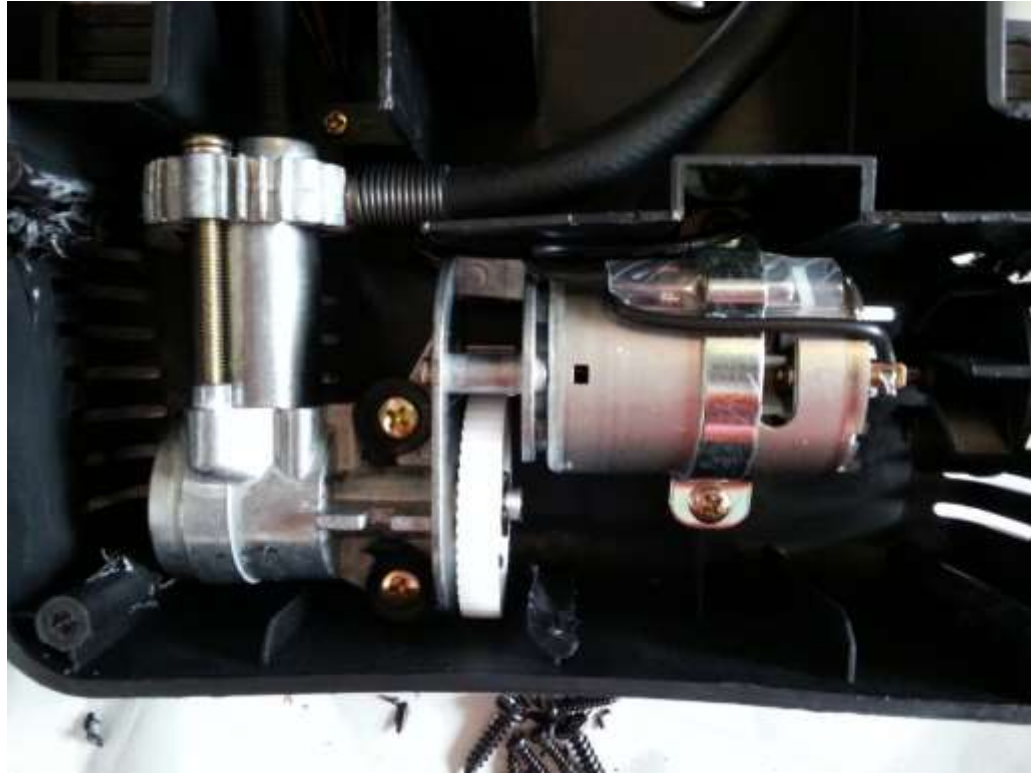
Fig. 174 – Inserting the motor/compressor assembly into housing
