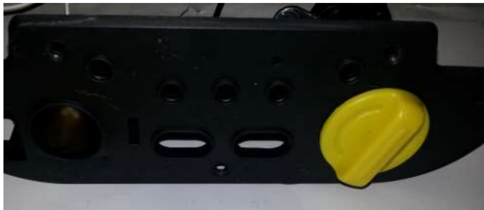
Fig 127 – Inserting the switch into front panel
