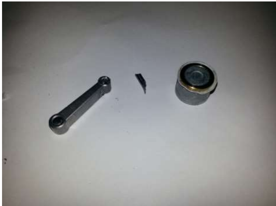
Fig. 119 - Attaching the piston to the crank arm
