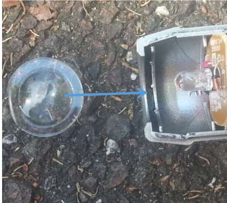
Fig. 149 – Inserting light diffuser
