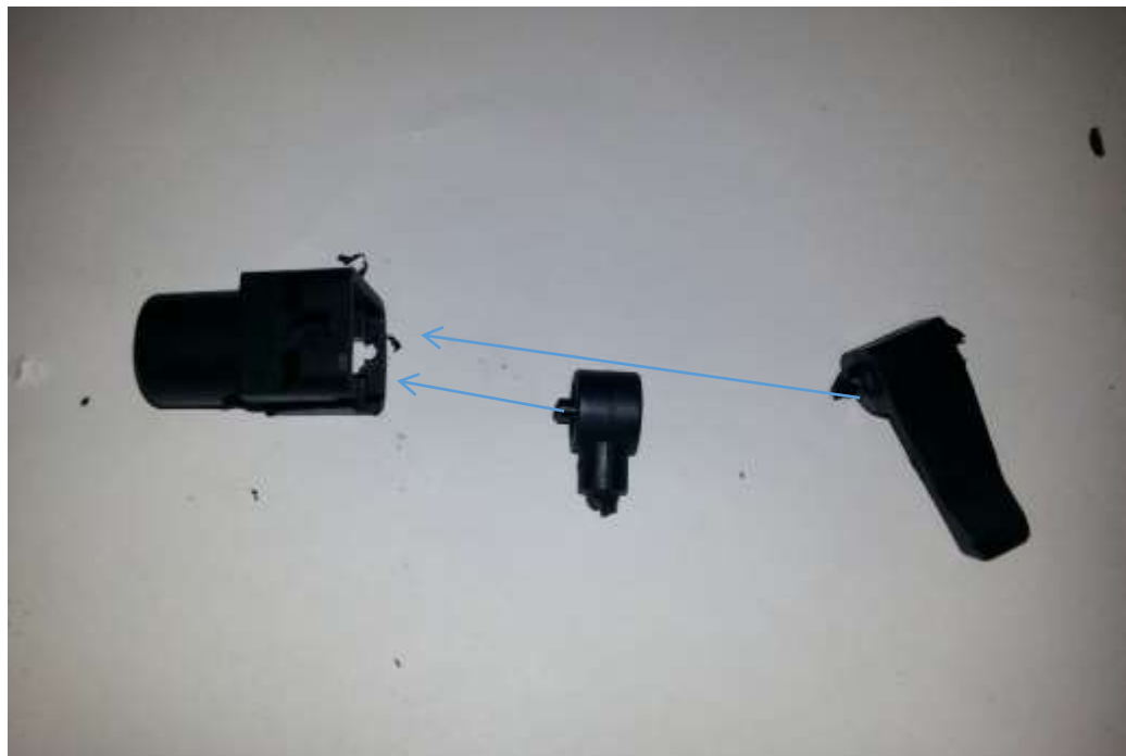
Fig. 95 - Assembly of the pump valve
