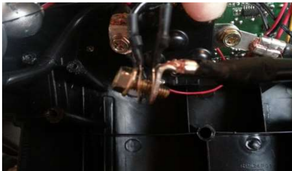
Fig. 156 - Attaching wires to the screw
