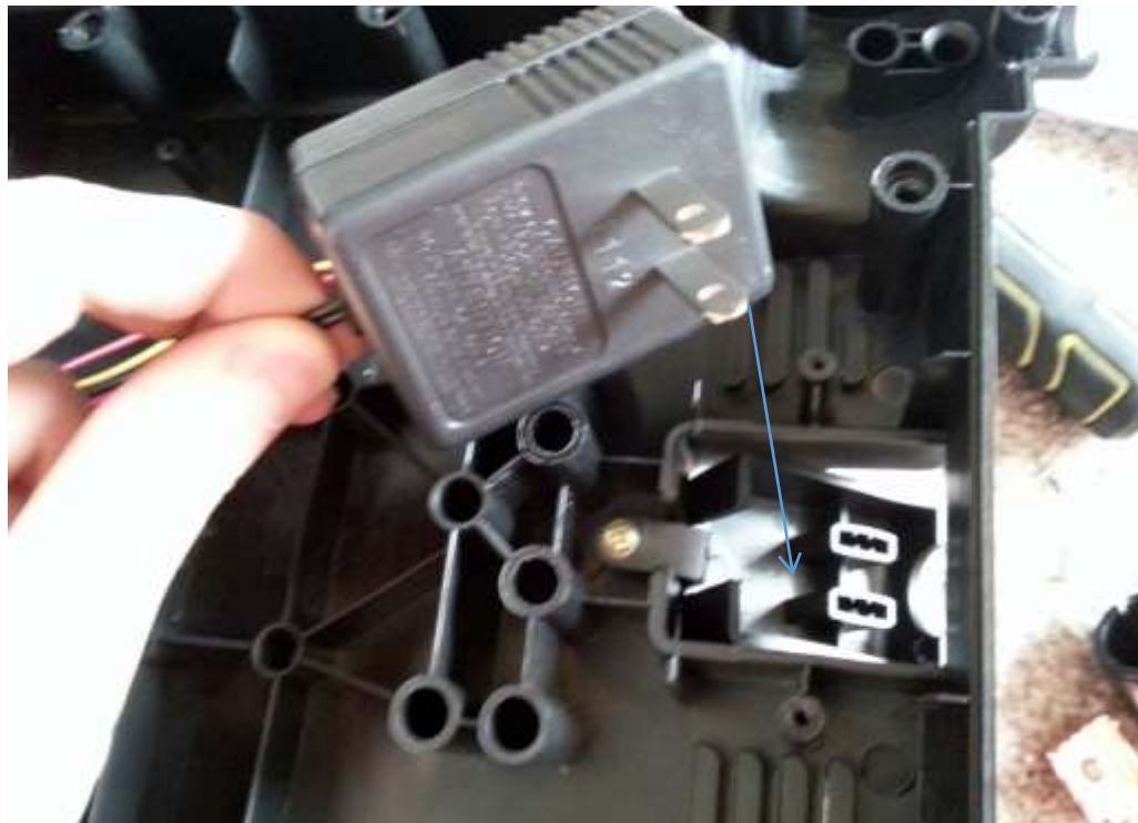
Fig. 164 - Inserting the AC adaptor
