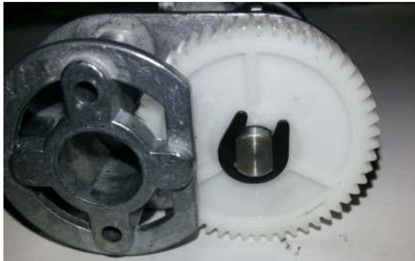
Fig. 117 – Fixing gear to the shaft
