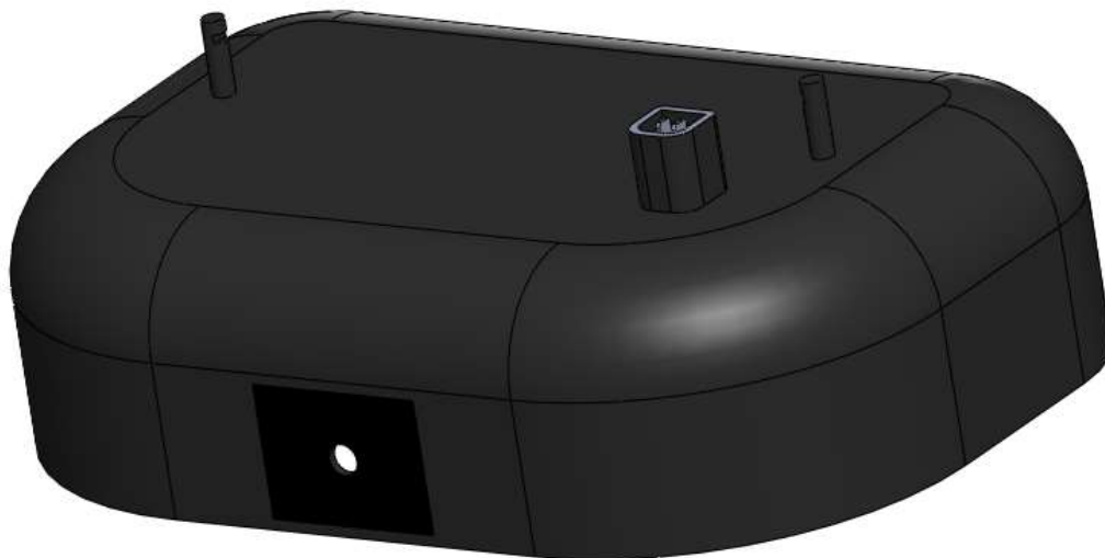
Fig. 65 –CAD model of the top part of the battery pack
