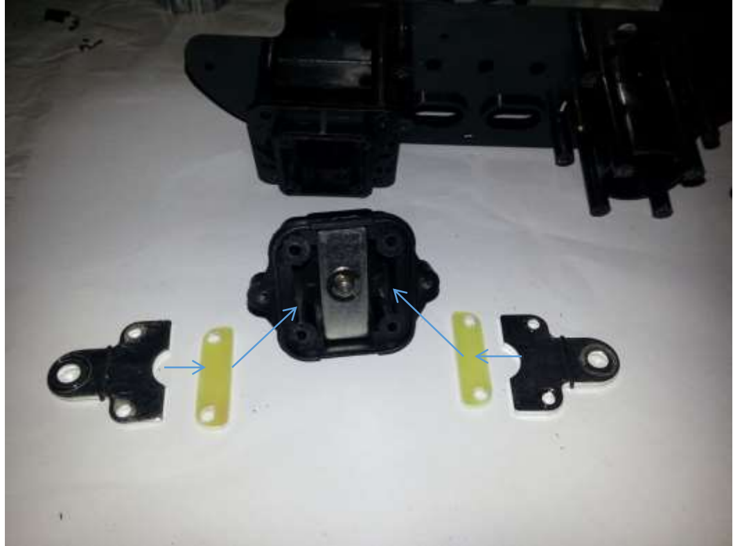
Fig. 136 - Inserting the space and metal brackets
