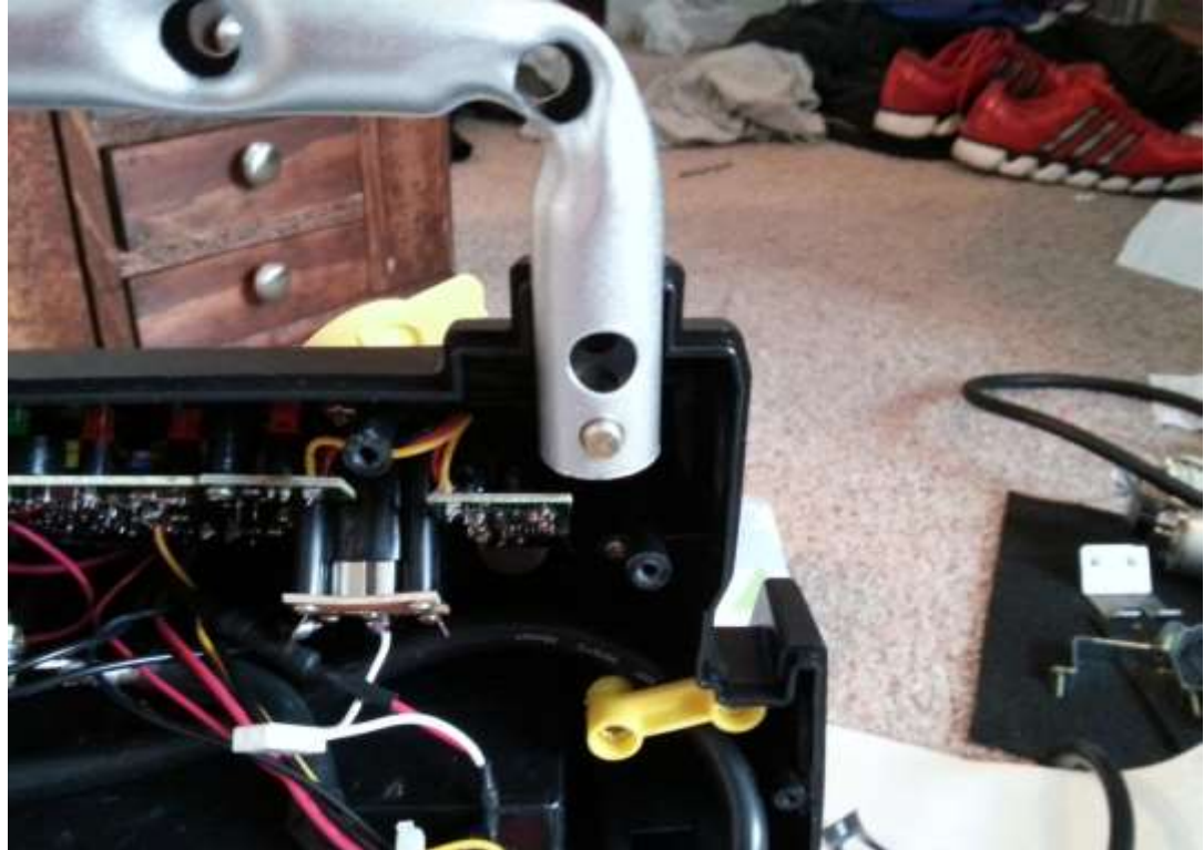
Fig. 166 - Attaching the metal handle to the housing
