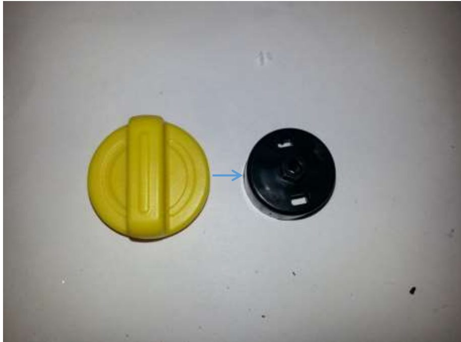
Fig. 126 - Attaching the on/off knob to the back piece
