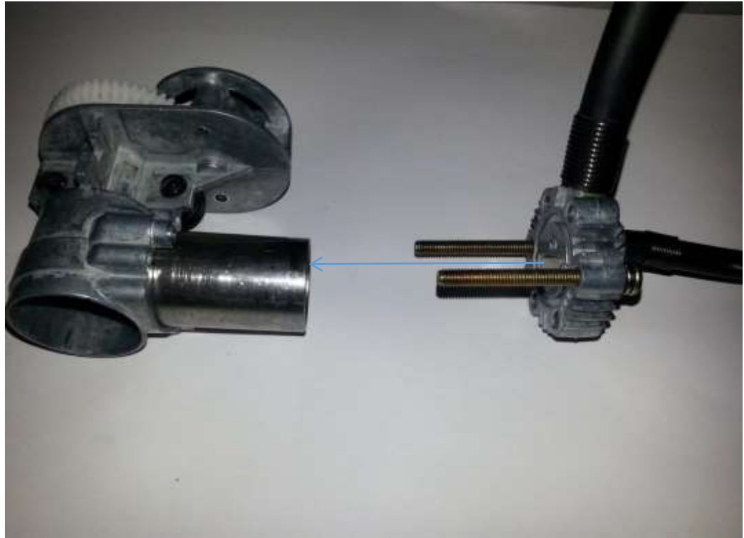
Fig. 122 - Attaching the top piece to the compressor
