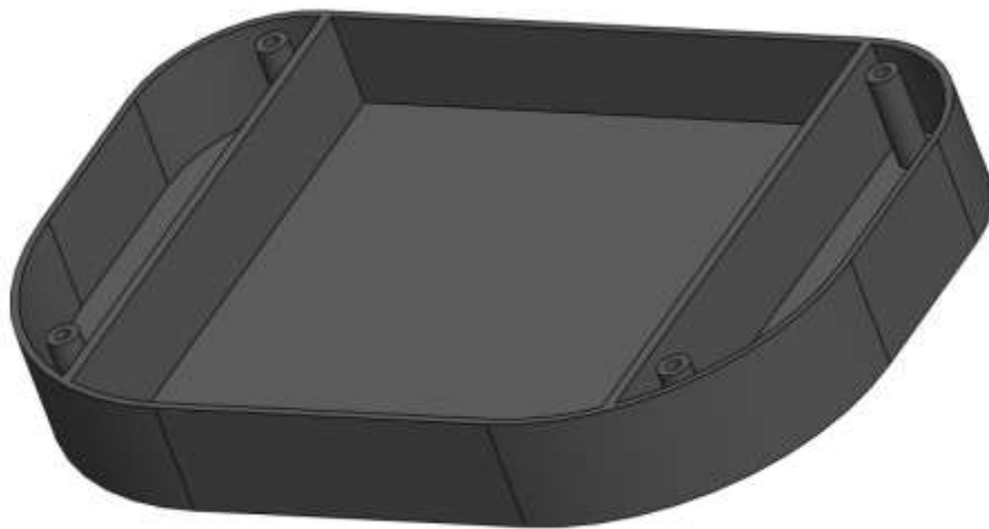
Fig. 64 – CAD model of the bottom part of the battery pack
