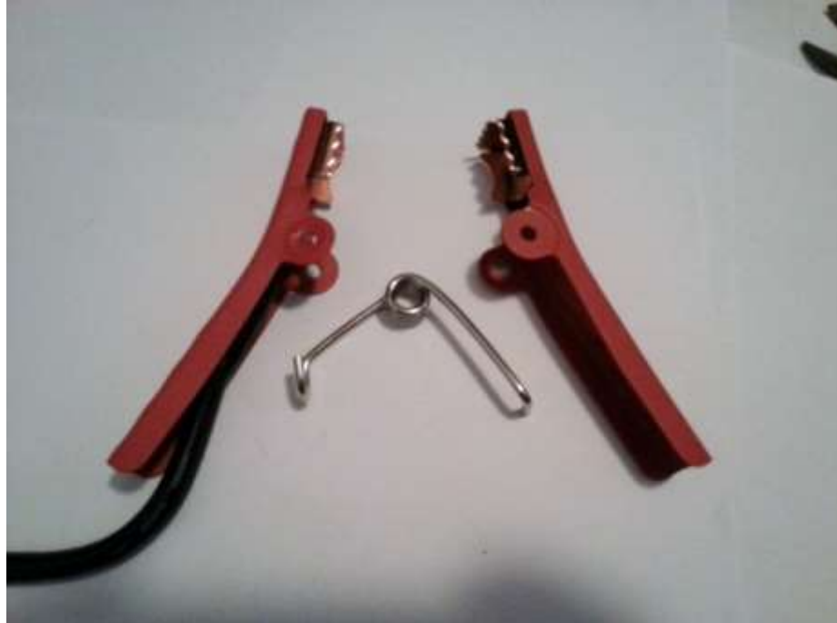
Fig. 182 – Aligning the spring between the two clamp halves
