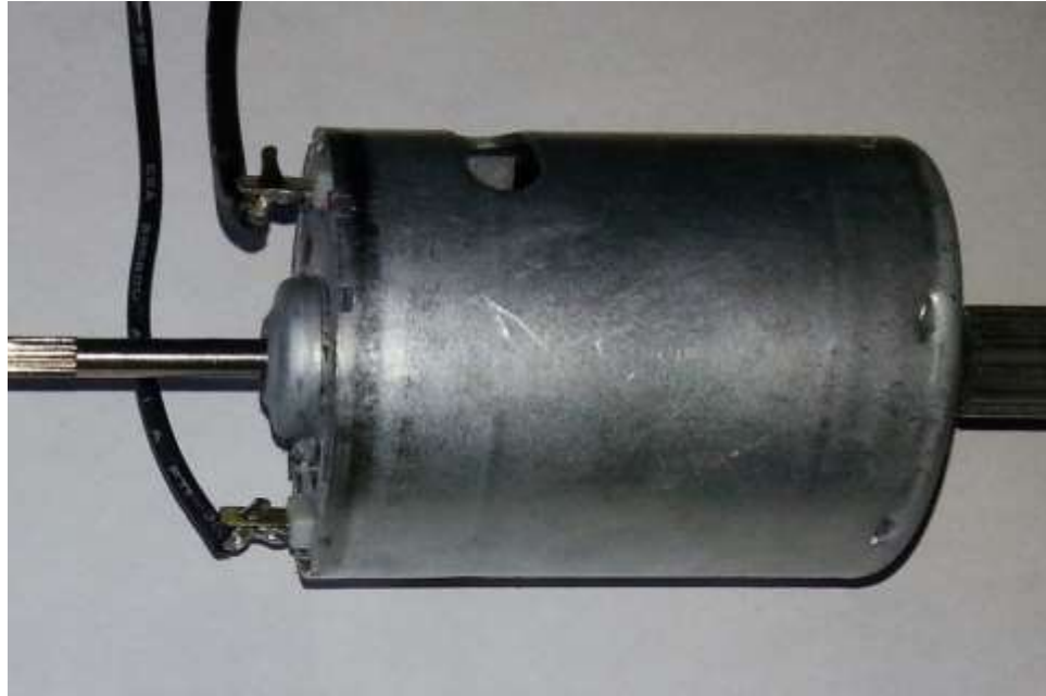
Fig. 172 – Soldering two wires to motor
