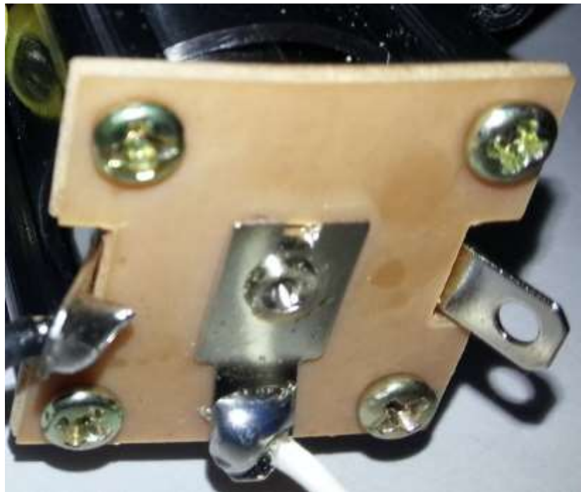
Fig. 141 – Attaching the backplate
