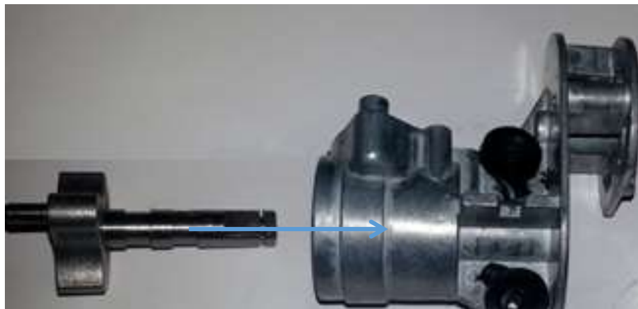
Fig. 115 – Inserting cam shaft into compressor housing
