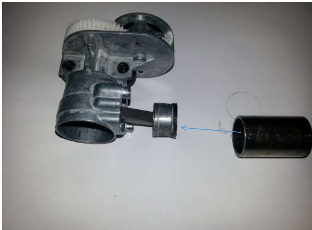
Fig. 121 – Placing the cylinder over the piston
