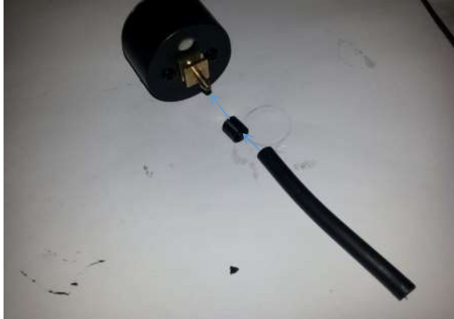
Fig. 112 - Attaching the pressure gauge to the hose
