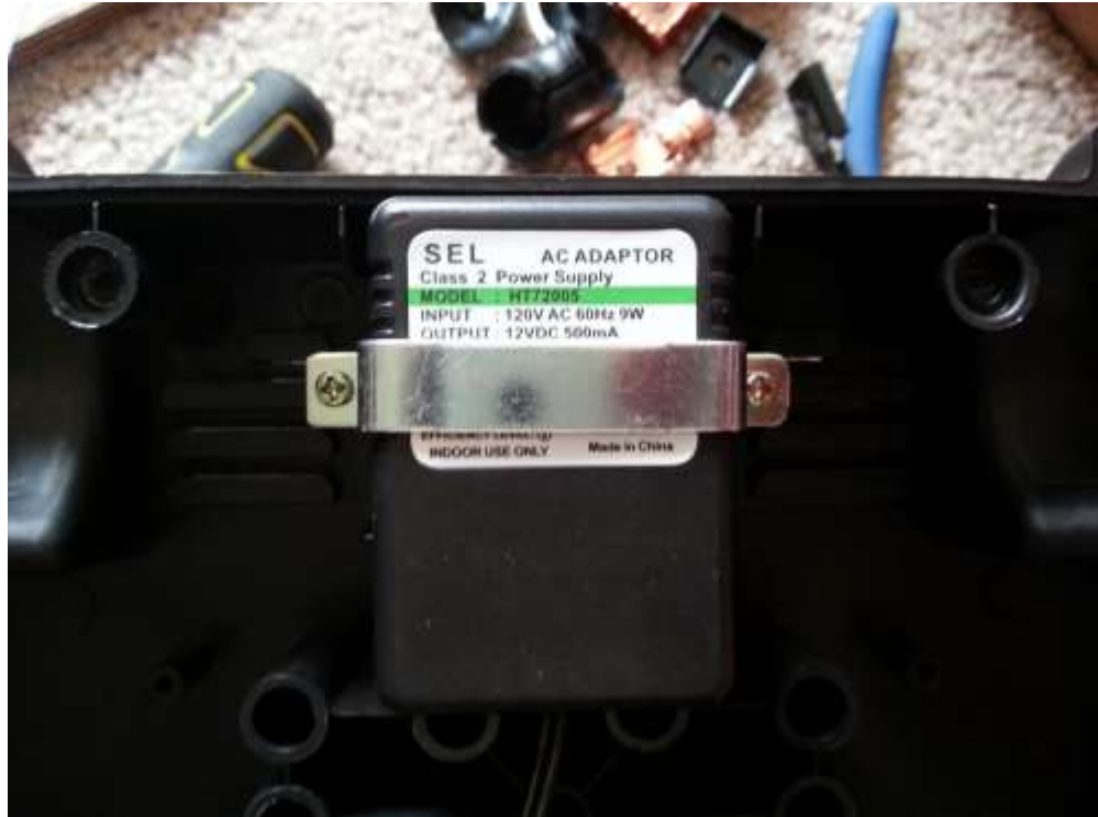
Fig. 165 - Securing the AC adaptor
