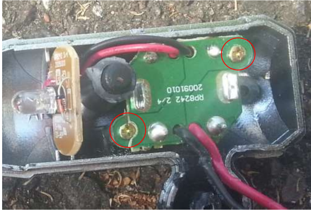
Fig. 148 – Attaching flashlight circuit board
