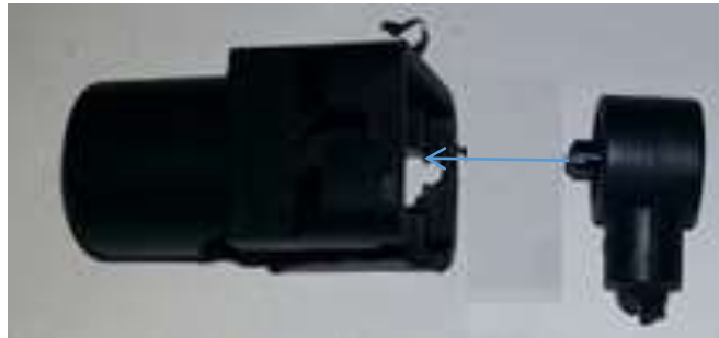
Fig. 94 - Inserting the Schrader valve into the housing
