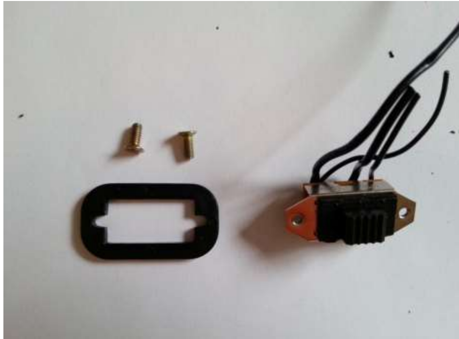
Fig. 169 – Solder wires on to switch
