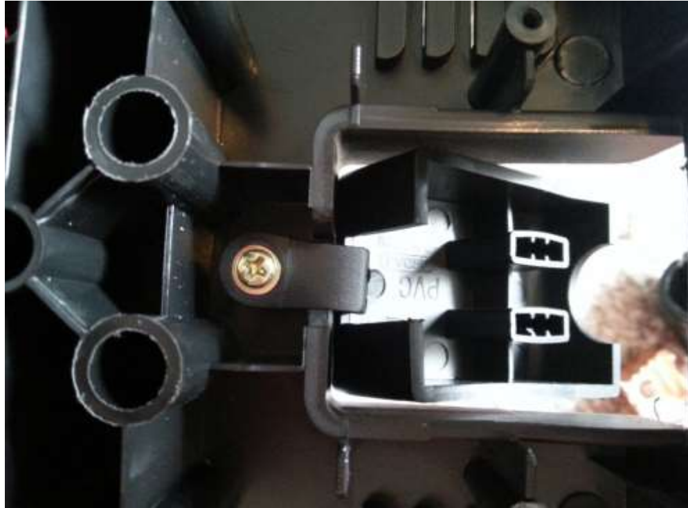
Fig. 163 - Attaching the AC adaptor cover
