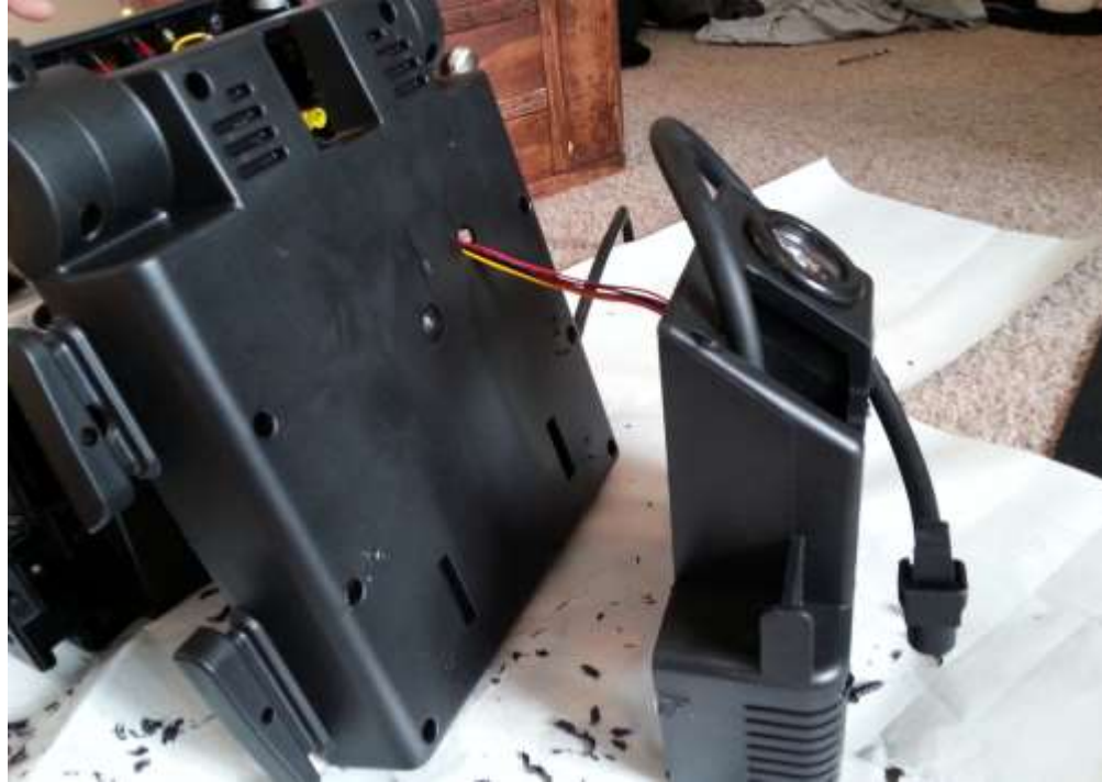
Fig. 167 - Pulling the wires through the housing
