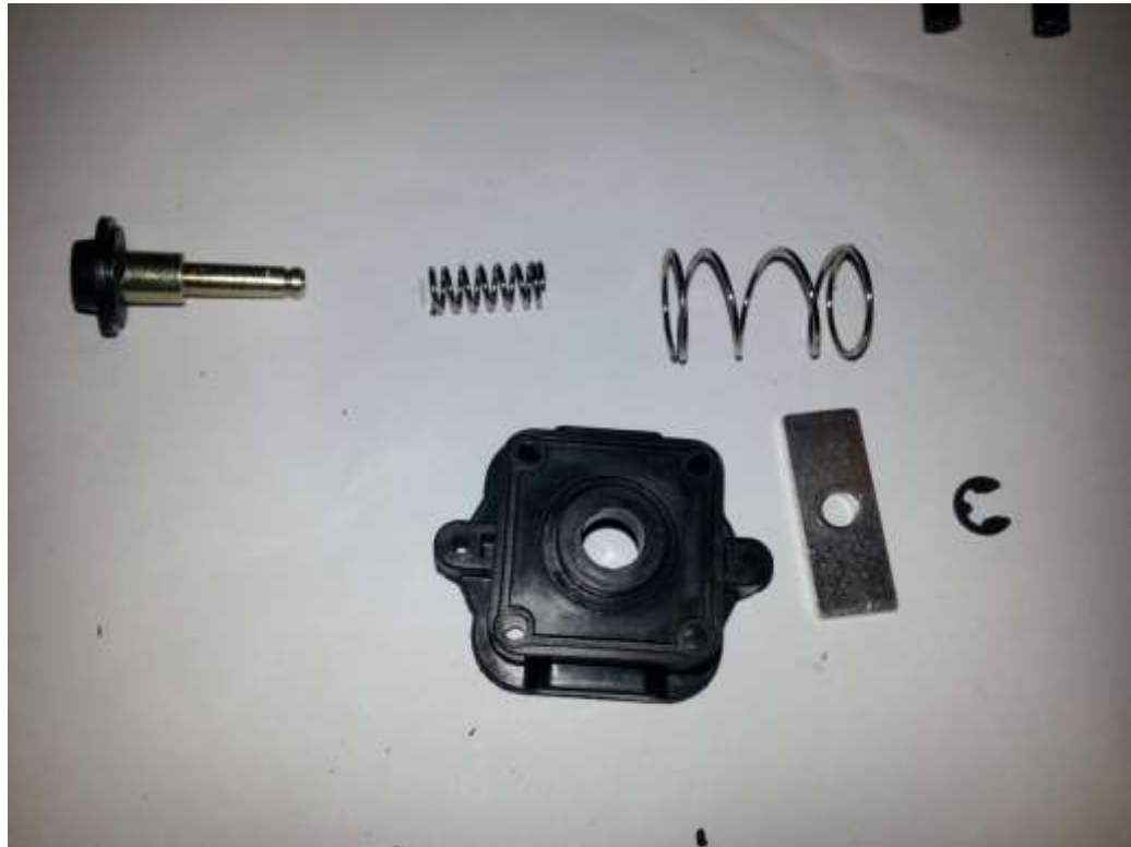
Fig. 131 - Preparing to assembly the middle portion of the on/off mechanism
