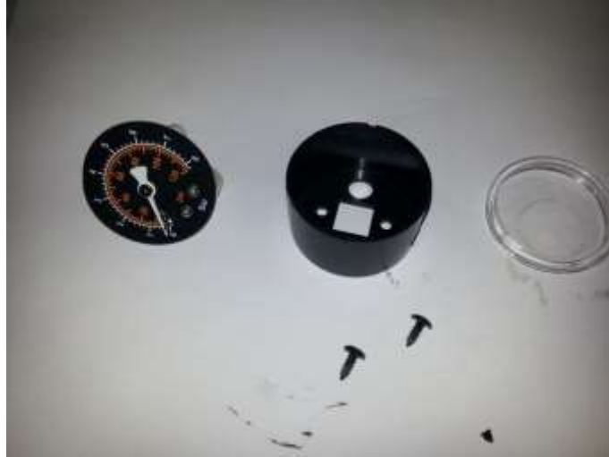
Fig. 110 - Preparing the pressure gauge assembly
