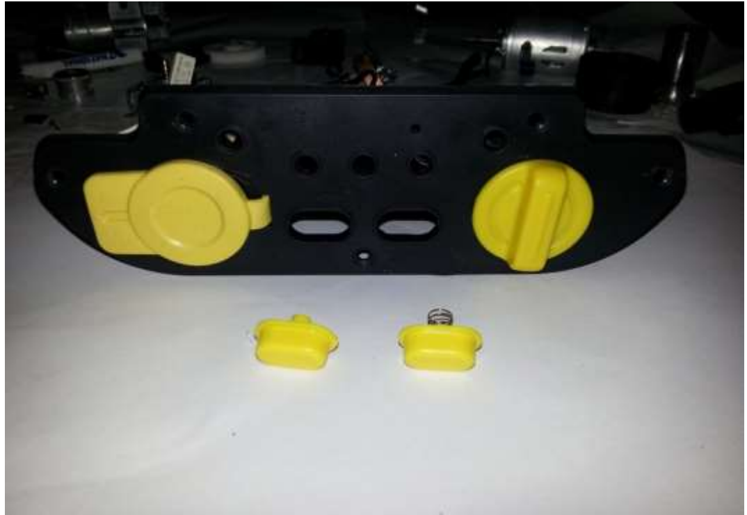
Fig. 146 - Inserting the buttons into the front panel
