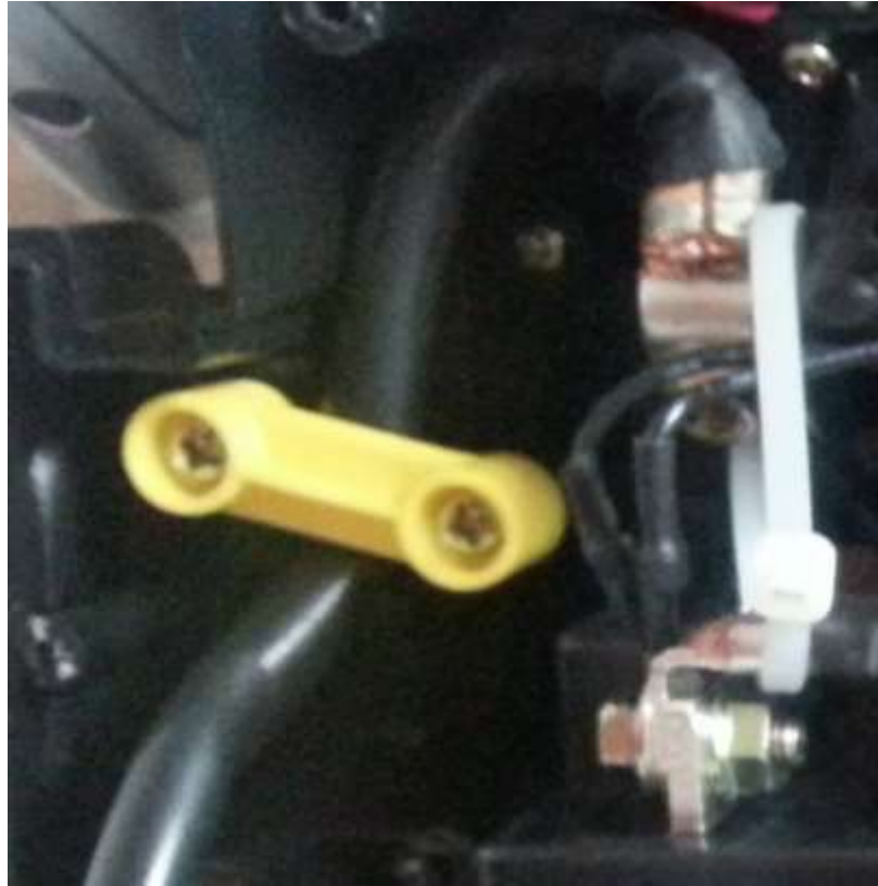
Fig. 160 – Arranging wire clamp # 1
