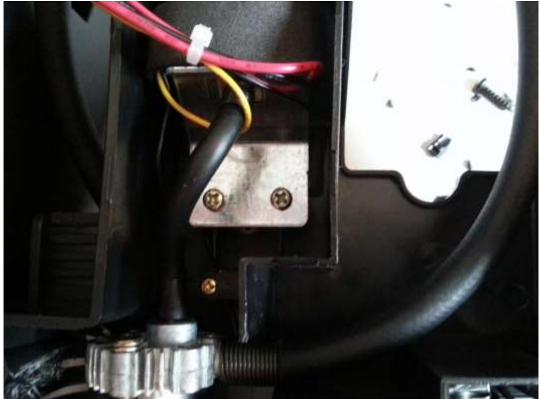
Fig. 175 - Attaching the bracket to hold the pressure gauge in place
