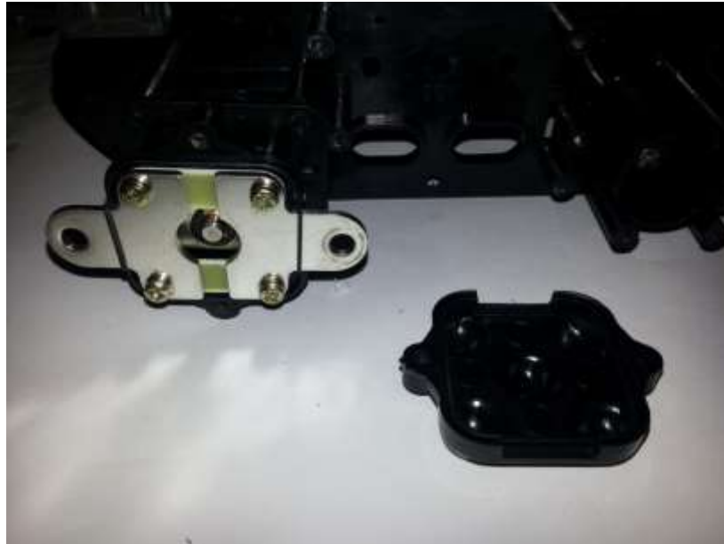
Fig. 137 - Attaching the back piece
