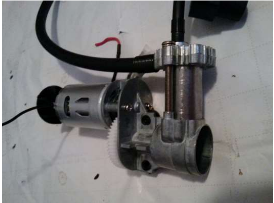
Fig. 125 - Full pump/compressor assembly
